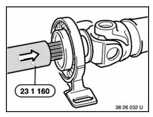
Drive on centre mount with ball bearing to fit tightly using Special Tool 23 1 160.
