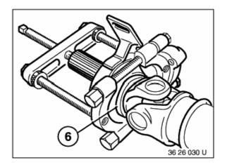
Apply Kukko puller on centre mount in such a way that dust cover (6) cannot be damaged.
