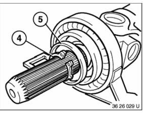
Lift out circlip (4).
