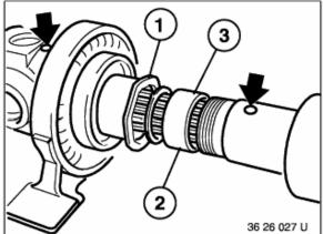
Pull off rear propeller-shaft section.
