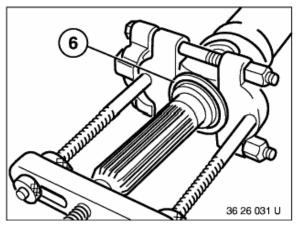
If dust cover was damaged (deformed), pull off dust cover with Kukko puller and replace.
